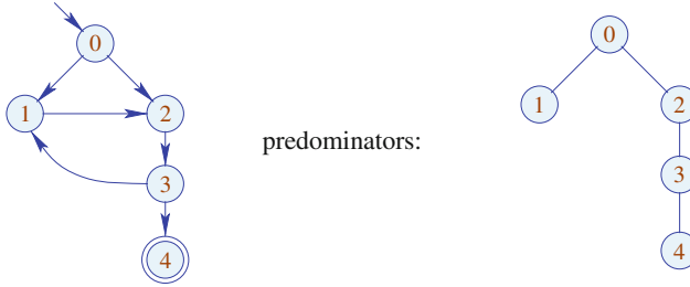
Fig. 1.56 A non-reversible loop
